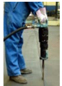
Try to keep the pick as near vertical as possible during operation
